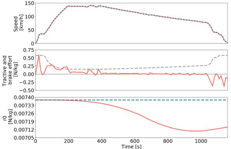
ukf can track speed measurements and estimate the running resistance parameters
