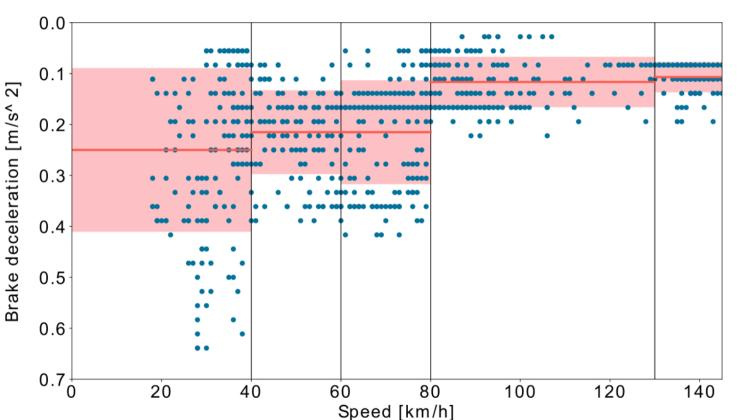
3 different brake rates along the 5 ATP braking speed steps
